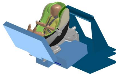
Rear impact, low pulse, deformed shell & headrest
