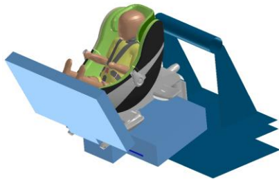
Frontal impact, medium pulse deformed shell & headrest
